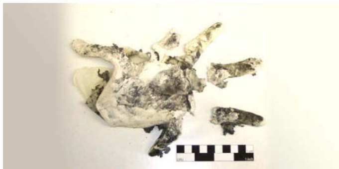
Figure 4-1. (top) 0.3g RBF trial, damage to dummy hand (Murray, et al, 2014)
