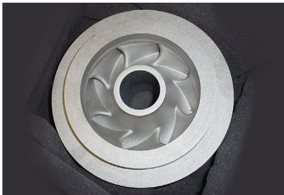
Figure 1: Impeller for Turbo Pump Made by PM HIP From Ti-6Al-4V Alloy (Source: LNT PM Inc.).
