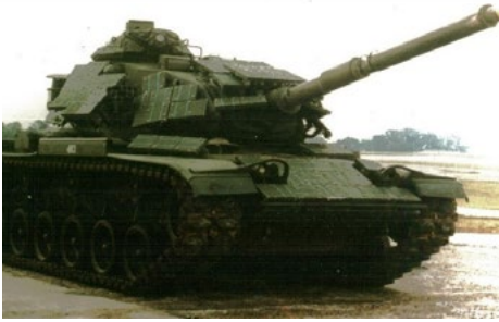
Figure 2: Reactive Armor Modules Containing ARL-Developed Technology Deployed on the Marine Corps' M60s Used in Desert Storm (Left) and the Abrams (Middle and Right) (Photos Courtesy of ARL and GDLS/PM Abrams).
