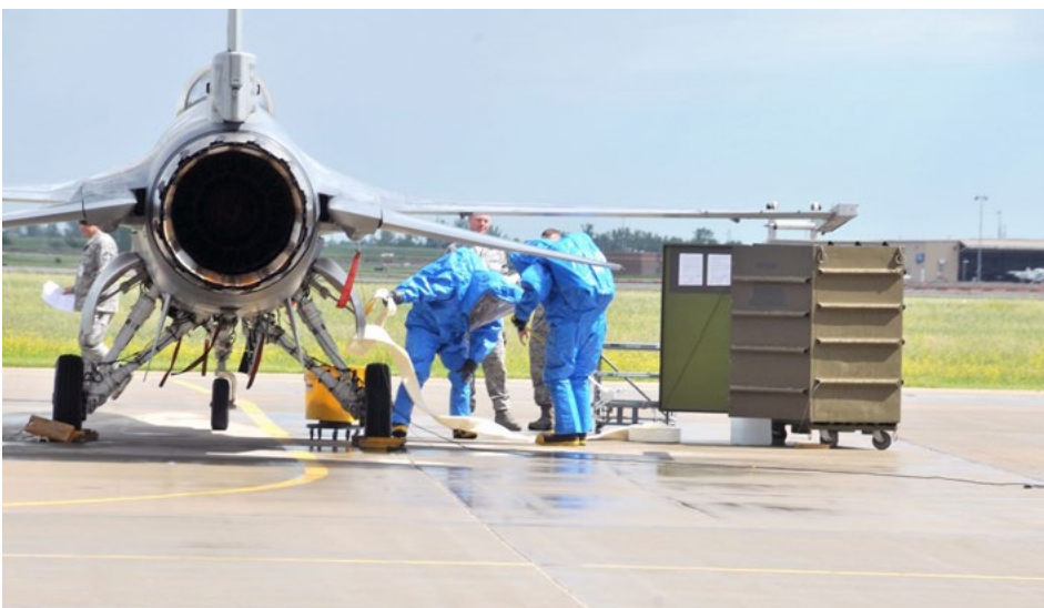
Figure 2: Members of a Hydrazine Response Team Use Protection to Prevent a Simulated Hydrazine Leak From Spreading (Source: Tech. Sgt. Christopher Stewart, National Guard [6]).
