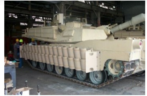
Figure 2: Reactive Armor Modules Containing ARL-Developed Technology Deployed on the Marine Corps' M60s Used in Desert Storm (Left) and the Abrams (Middle and Right) (Photos Courtesy of ARL and GDLS/PM Abrams).
