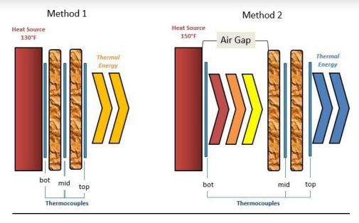
Figure 7: Thermal Transmission Test Methods (Source: QNA).
