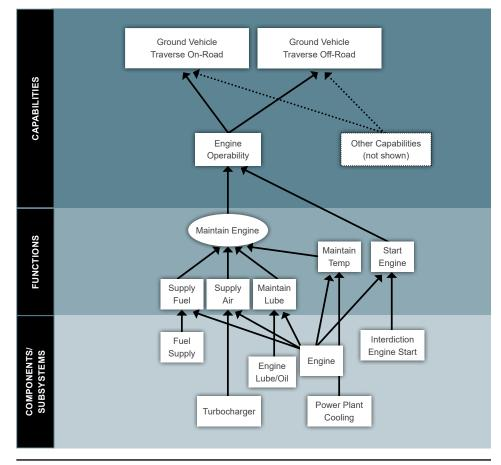
Figure 1: Simplified Functional Tree for Ground Vehicle Traverse (Source: Andrew Drysdale).
