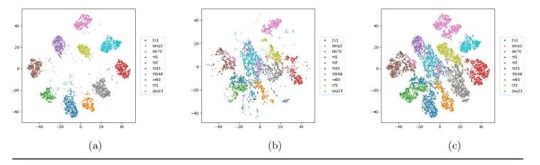
Figure 3: A Two-Dimensional Visualization of the Measured (a) and Synthetic (b) Portions of the Dataset, Along With Two Portions in One Graph (c) (Source: AFRL).
