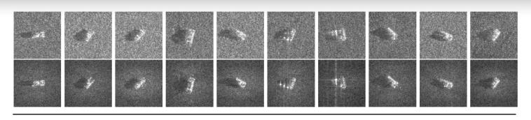
Figure 2: Randomly-Chosen Images of Each Vehicle in the SAMPLE Dataset, With Measured (MSTAR) Images (Top Row) and Corresponding Synthetic Images (Bottom Row). The Order of the Vehicles From Left to Right Matches Table 1 (Source: AFRL).
