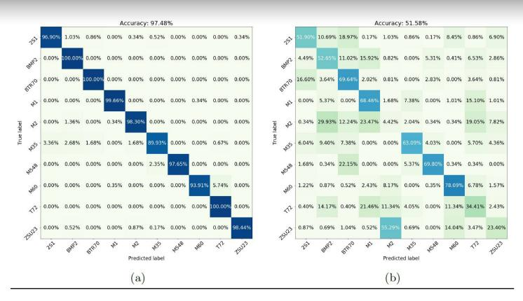
Figure 4: Confusion Matrices for a DenseNet Network Trained and Tested on Measured Data (a) and Trained on Synthetic Data and Tested on Measured Data (b) (Source: AFRL).
