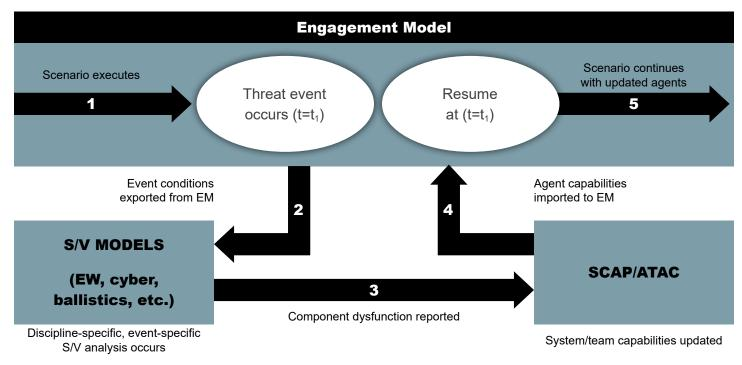
Figure 4: Integration of SCAP/ATAC With Component SVL and Engagement Models (Source: Andrew Drysdale).
