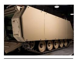
Figure 10: Prototype ARDDM Kit Integrated Onto M113 Troop Carrier (*Source: QNA*).
