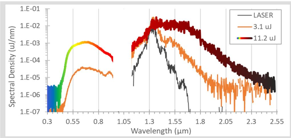
**Supercontinuum in Sapphire Glass With 1.3  $\mu\text{m}$  OPA Source**
