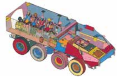
Figure 3: High-Fidelity Finite Element Model of an Example Vehicle (Source: ARL).
