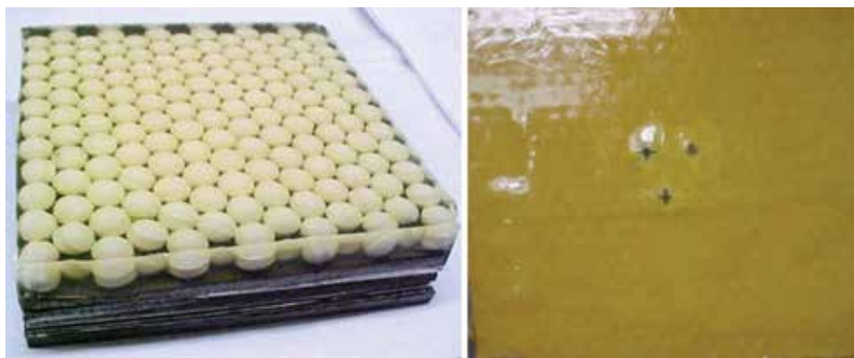
Figure 3: Ceramic Spheres Embedded in Elastomer (Left); Front-Side After Penetration by Three 0.50-cal. AP Rounds Falling Within 2-inch Circle (Stanag 4241 Bullet Impact Test), Showing Small Holes in Kevlar Top Layer (Right). The Damage Zone Is Less Than the Bullet Diameter Because the Elastomer Contains the Ceramic Granulated by the Projectile (Source: NRL).
