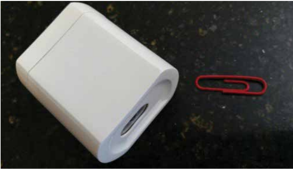
Figure 3: Example of a COTS Pocket-Sized Spectrometer for Authentication (Source: InfraTrac ).
