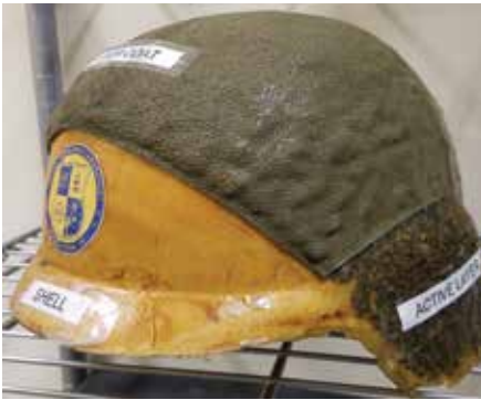
Figure 5: Advanced Combat Helmet Core With Added Layer of Resonating Elastomer Containing 33% Hollow Spheres. The Latter Have the Same Density as the Polymer, So the Helmet Weight Is Independent of Sphere Content (Source: NRL).
