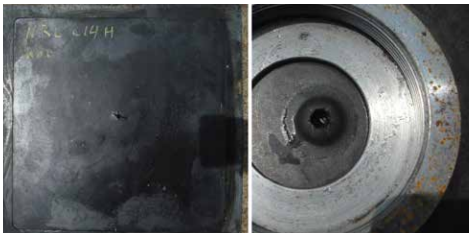
Figure 4: Elastomer Coating on Front of Steel Tank After Penetration by .50-cal. AP Round (Left); Hole in Center Has Completely Closed; Backside of Steel Vessel, With Hole Approximately 50% Larger Than Bullet Diameter (Right) (Source: NRL).
