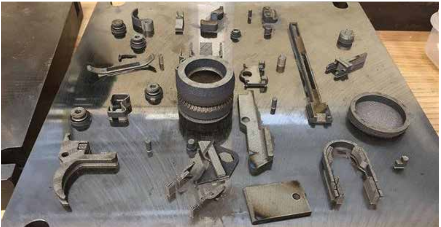
Figure 2: R.A.M.B.O.'s 3-D-Printed Parts (Minus the Receiver and Barrel) (Credit: U.S. Army ARDEC, Source: http://asc.army.mil/web/news-alt-amj17-rambos-premiere/ ).
