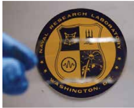
Figure 6: Transparent Elastomer Used for Coating (Source: NRL).
