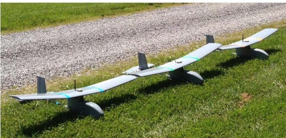
Figure 5: Model Planes Used as Surrogate for Raven RQ-11.
