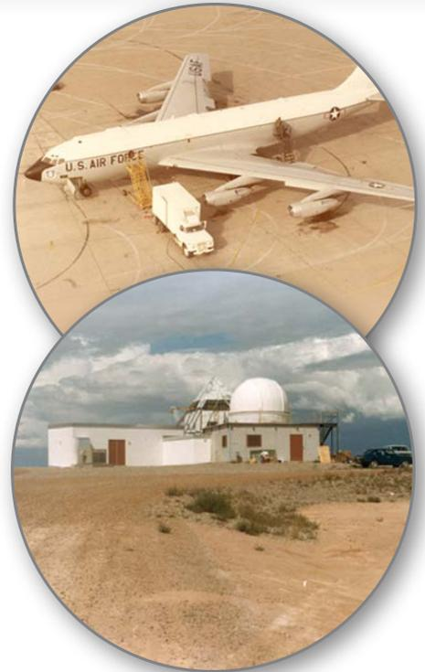
Figure 1: Airborne and Ground Terminal Platforms for the AFTS Demonstration at White Sands Missile Range, NM. Top: Airborne High-Data-Rate Transit Terminal Installed in KC-135 (With Ground-Based Test Equipment); Bottom: Airborne High-Data-Rate Ground Station Receiver Located at Cowan Site [3].
