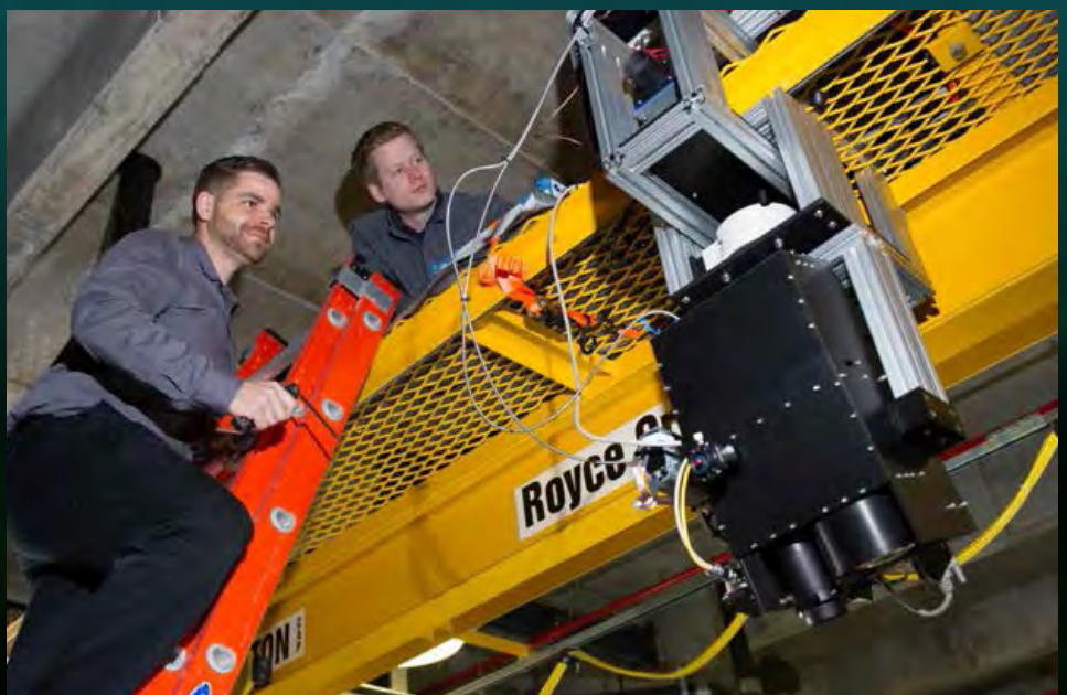
Figure 1: The GTRI Lightweight Lidar Prototype Gantry-Mounted Over a Laboratory Water Tank.
