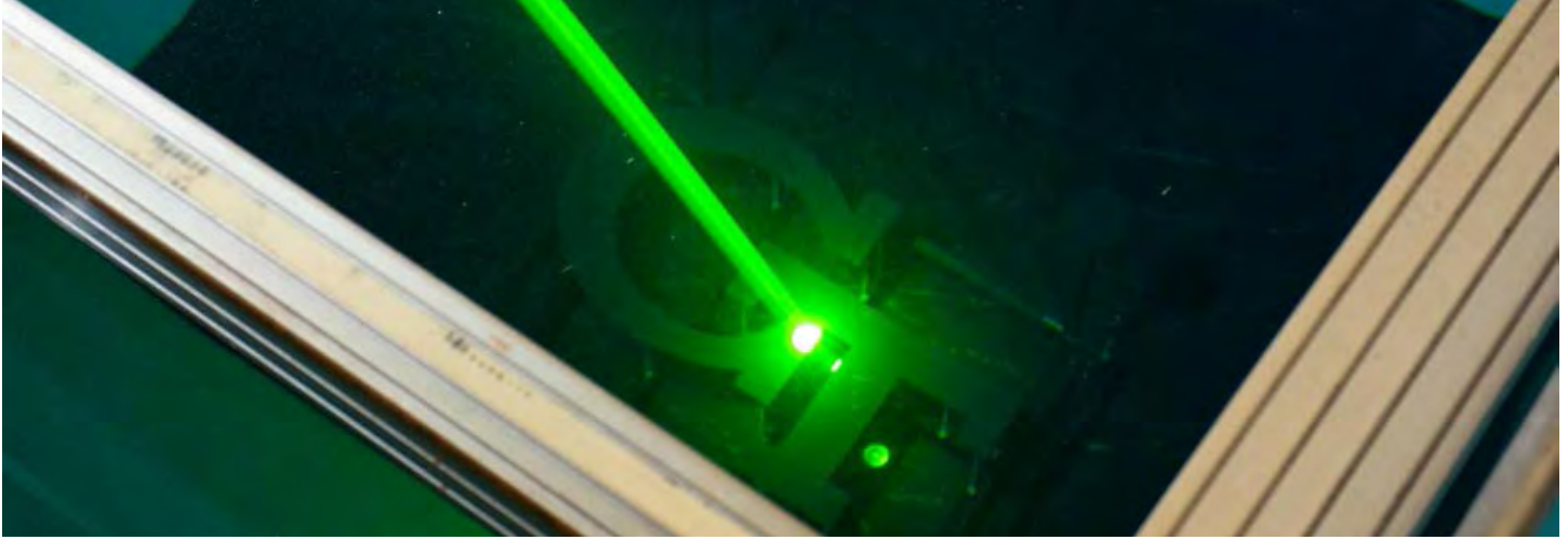
Figure 2: The Special Green Laser of GTRI Lightweight Lidar Prototype System Used to Penetrate Water and Help Researchers Study the Best Methods for Producing Accurate Images of Objects on the Pool Floor.
