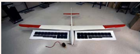
Figure 3. COTS Glider With Monocrystalline Silicon Photovoltaic Cells (NRL Photo).
