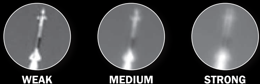
Figure 1: The Effect of Different Strength Turbulence on the Image of a Rocket.
