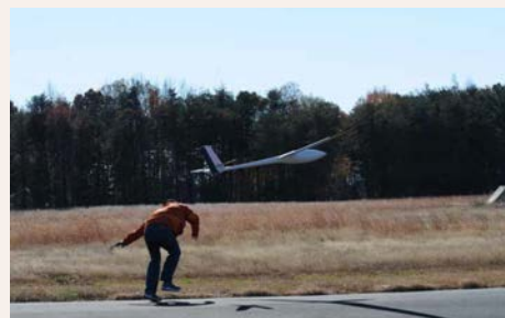
Figure 4 (top): Flight Data Illustrating ALOFT Gaining 1,500 ft of Altitude in a Thermal Updraft. The Warmer Colors Indicate Higher Climb Rates. Figure 5 (bottom): Hand-Launching a Powered Sailplane UAV to Test the Autonomous Soaring Algorithms (NRL Photo).
