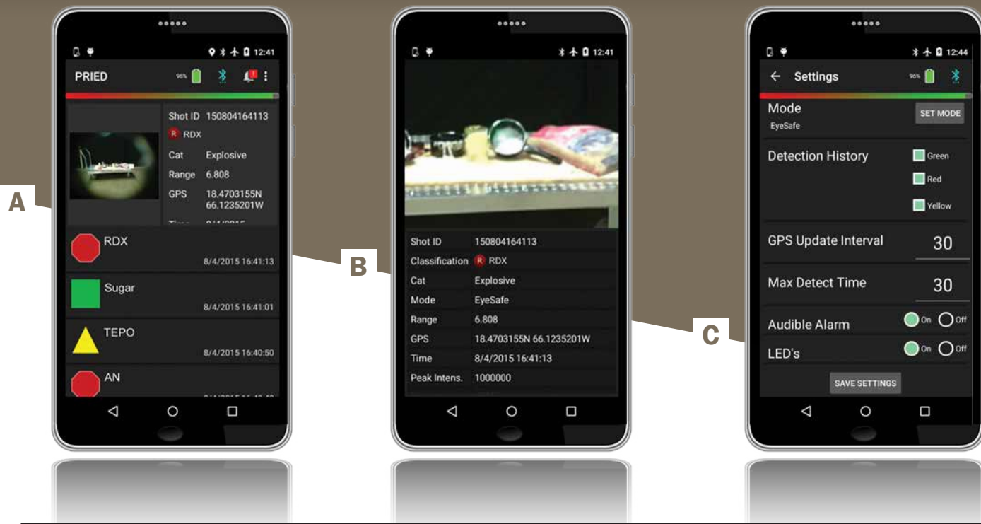
Figure 2: PRIED Android Application (a) Measurement History, (b) Measurement Details With Zoomed-In Image of Sampled Location, and (c) System Settings.
