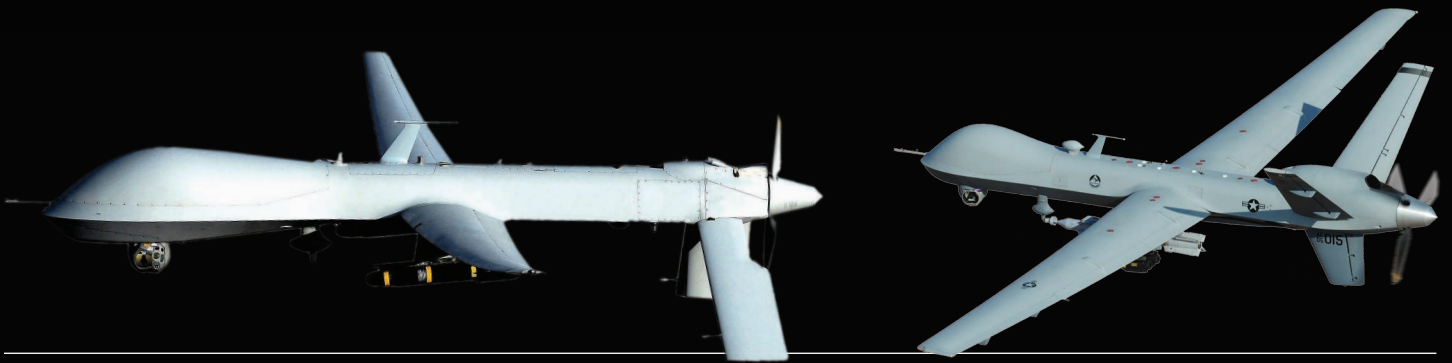
Figure 1: An MQ-1 Predator (Left) and MQ-9 Reaper (Right), Which Provided Intelligence, Surveillance, and Reconnaissance During Operation Iraqi Freedom (OIF) and Operation Enduring Freedom (OEF) (U.S. Air Force Photo/Lt. Col. Leslie Pratt).
