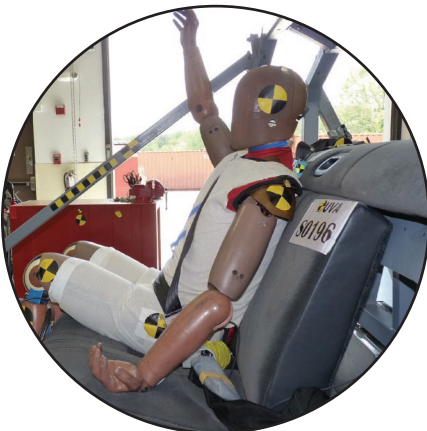
Figure 4: ATDs in a Vehicle to Simulate/Measure Human Occupant Responses (University of Virginia, National Highway Traffic Safety Administration).
