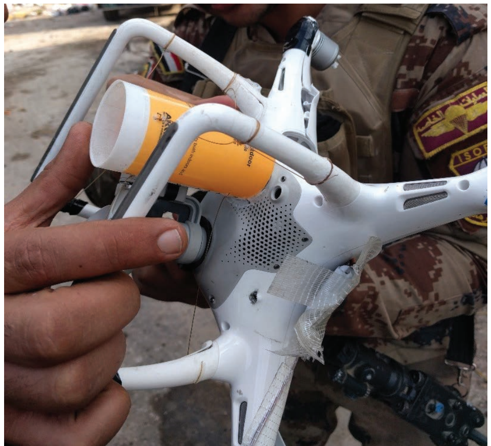
Figure 1: Iraqi Counter Terrorism Forces Examine an ISIS Drone Modified to Drop Small Explosives (Photo Courtesy of Mitch Utterback).
