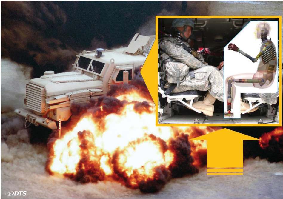
Figure 7: The Highly Vulnerable Leg in UBB Events (Photo Courtesy of the U.S. Army and Diversified Technical Systems Inc.).
