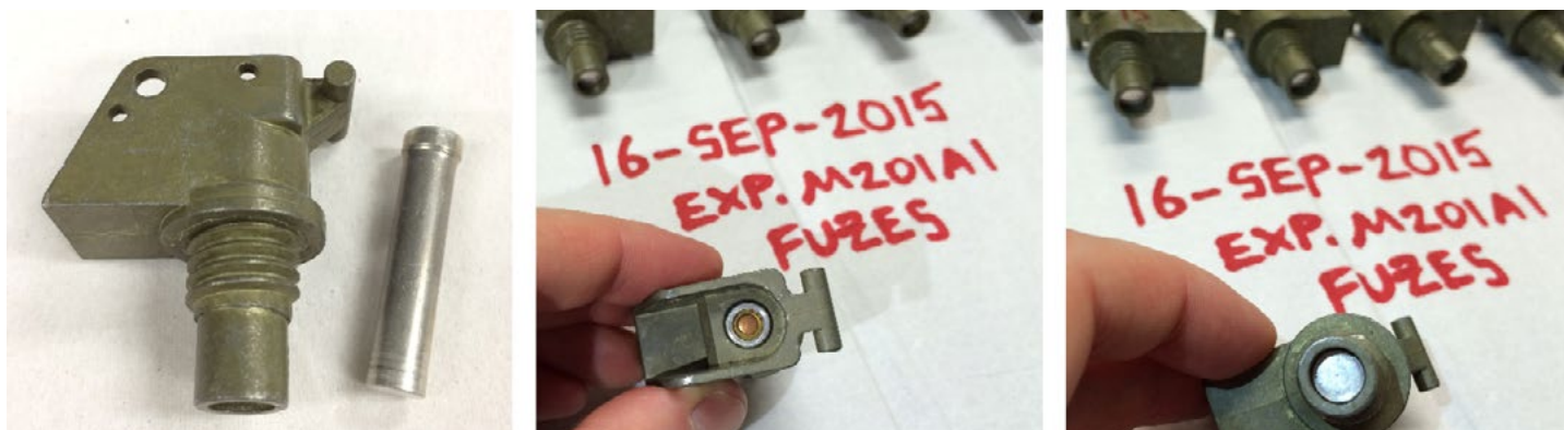
Figure 5: An M201A1 Fuze Body and Delay Case (Left), Top of an Assembled Fuze Showing the Primer (Middle), and Bottom of an Assembled Fuze Showing the Closed End of the Delay Case (Right) (Source: CCDC Armaments Center).
