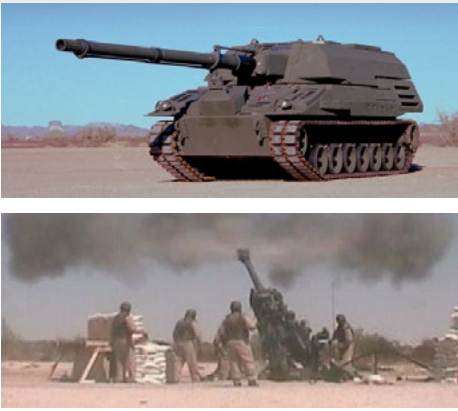
Figure 5: Two Artillery Systems Modified for Laser Ignition: The Crusader (Top) and LW155 (bottom) (Source: G. Burke).
