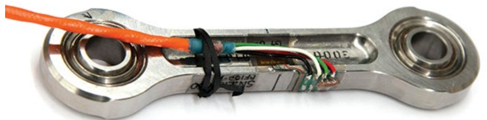
Figure 5: Titanium Link and Fitting Assembly for the V-22 (Source: Noel Hepp, U.S. Navy).
