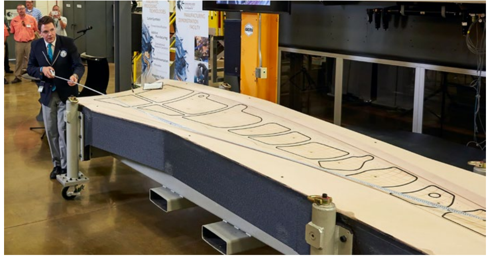
Figure 3: One of the Largest AM-Produced Parts in the World (Source: Oak Ridge National Laboratory).
