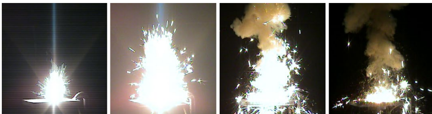
Figure 4: Open-Air Combustion of a 1.5-g Pellet of IC-5 (Source: CCDC Armaments Center).
