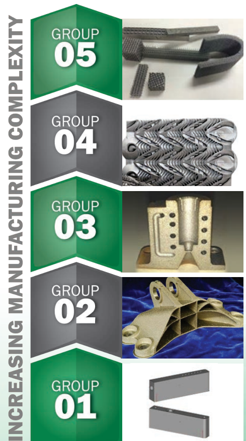
Figure 2. Examples of the Increasing Complexity in Design That AM Allows.
