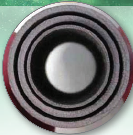
Figure 1. Titanium "Tube in a Tube" for a Cryo-Thermal Switch on ASTRO-H. Traditional Manufacturing Would Cost up to $20,000 and Take 3 Months to Build, While AM Can Drop the Cost to $1,200 and the Wait Time to 2 Weeks [4].
