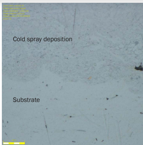
Figure 9: Section Through One of the Small Samples Shown in Figure 8 Exhibiting Mechanical Mixing at the Interface of Deposition and Substrate (Source: ARL).
