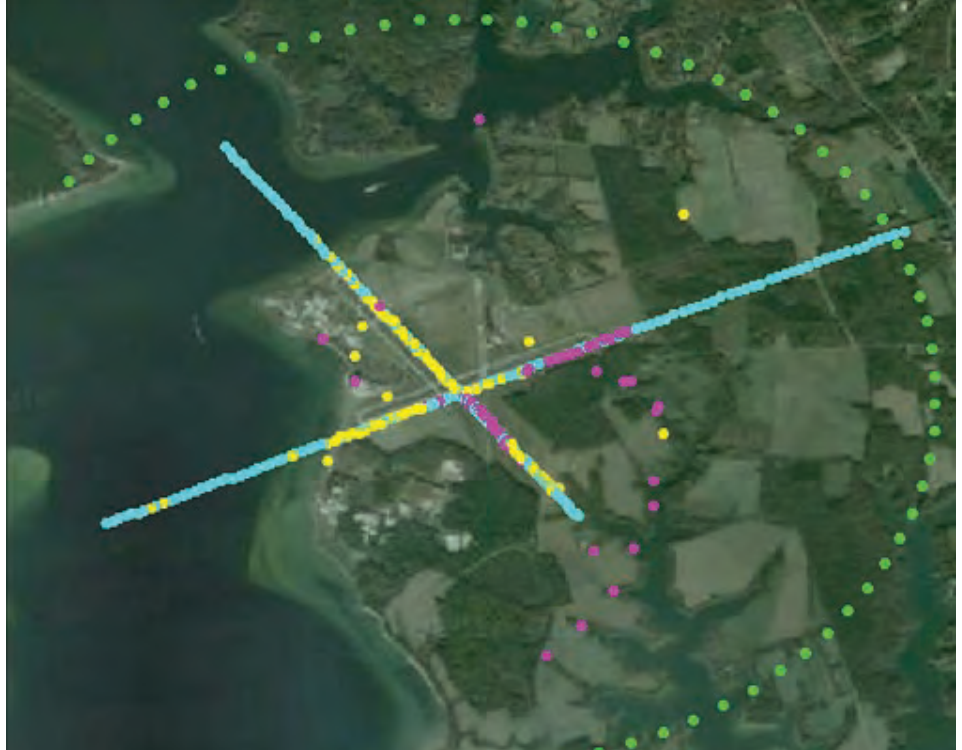
Figure 1: Scenario 1 - Radar Detections, Truth Data, and Platform Position Overlaid on a Terrain Map.
