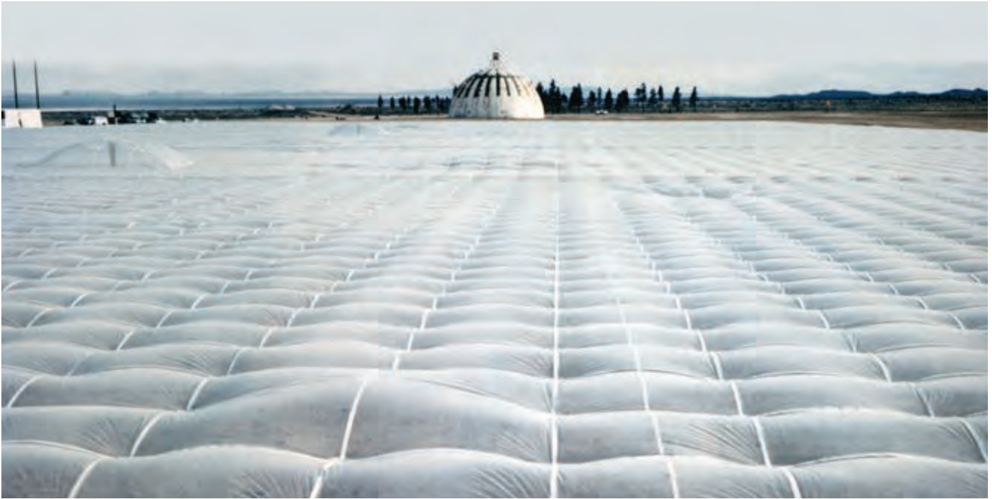
Figure 14: Misty Picture Test Bed Showing HE Source (in Background) and Mylar Helium Bag.
