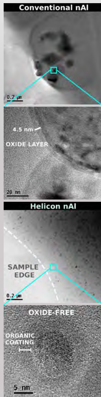
Figure 3: Comparison of In Situ nAl With Conventional Micron Aluminum in HTPB [10].
