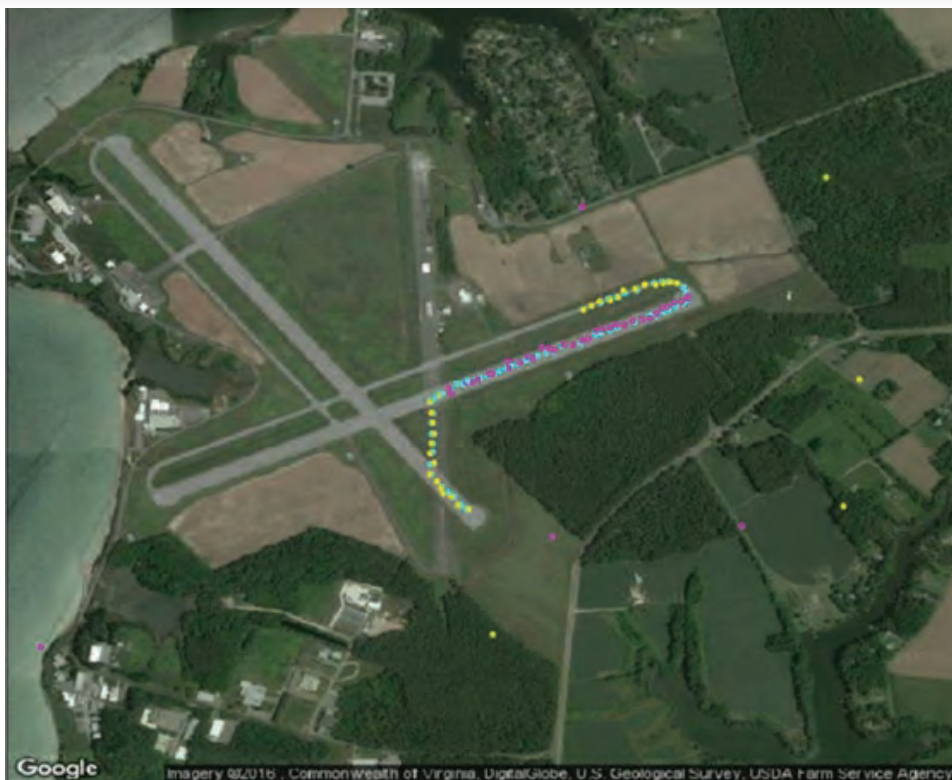
Figure 3: Detections (Shown in Magenta and Yellow) and Truth (Shown in Cyan) for a Single Vehicle.
