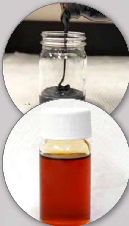
Figure 2: In-Situ-Produced nAl in HTPB (top) and \text{nTiO}_2 in HTPB (bottom) [10].
