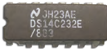
Figure 3: A Partially "Blacktopped" and Stamped Part With a False Identification Code. Part Number indicates a CLCC Package, but This Package Is a CDP. (NASA)
