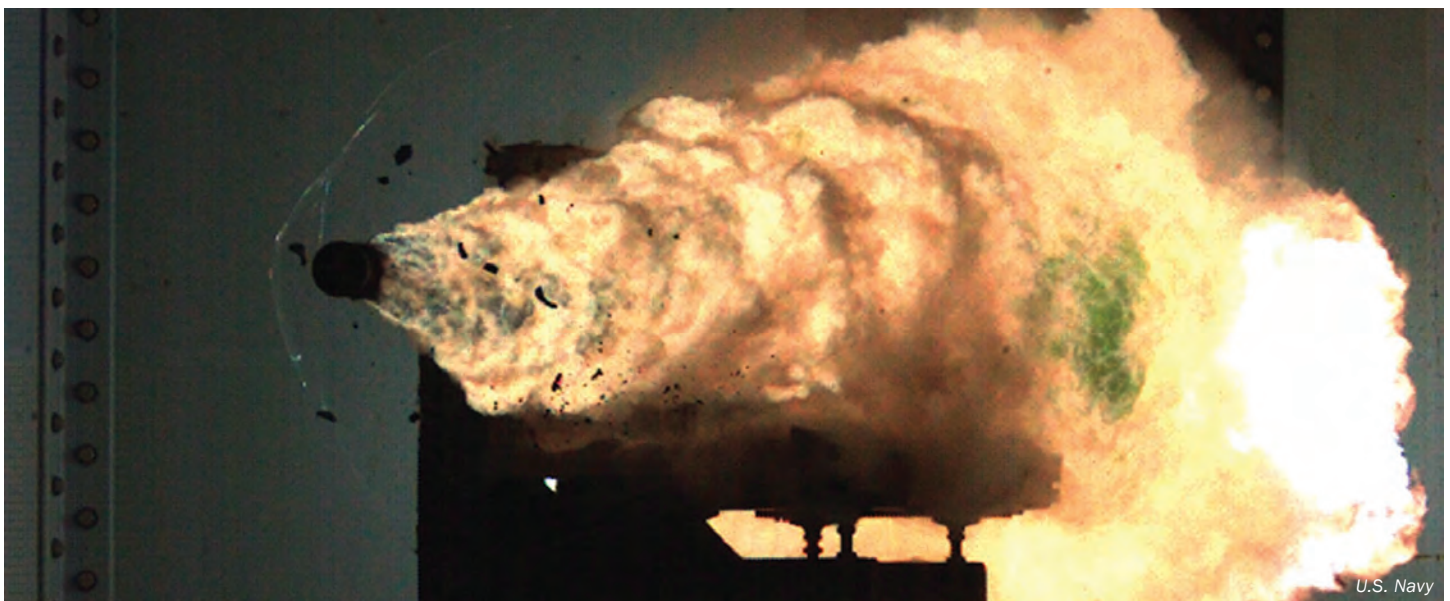
Figure 2: High-Speed Photo of Record-Setting Firing of NSWC Dahlgren's EMRG.
