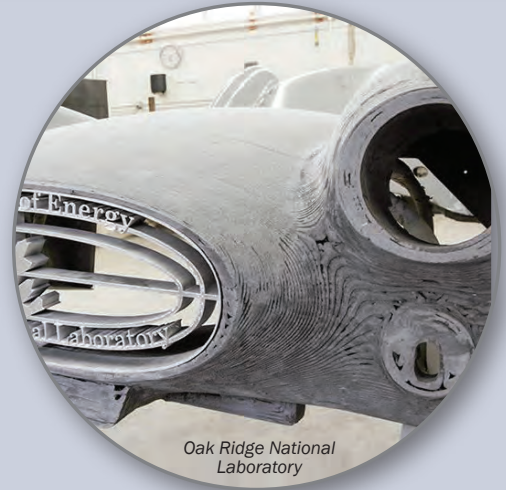
Figure 1 (above and below): 3-D Printed Car Produced at the Manufacturing Demonstration Facility, Oak Ridge National Laboratory (ORNL).
