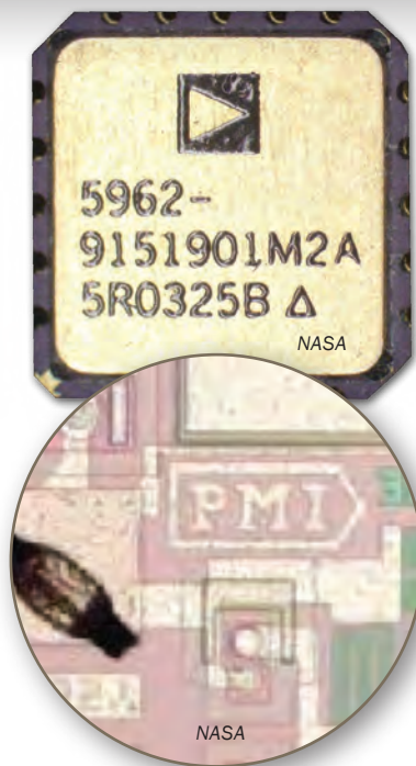
Figure 4: A Part with Falsified Function Markings. The Markings (top) Indicate an Op Amp From ADI, but the Part Contains Die from a Voltage Reference From PMI (bottom).
