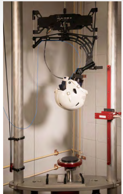
Figure 2: Chesapeake Testing's Twin-Wire Drop Tower.
