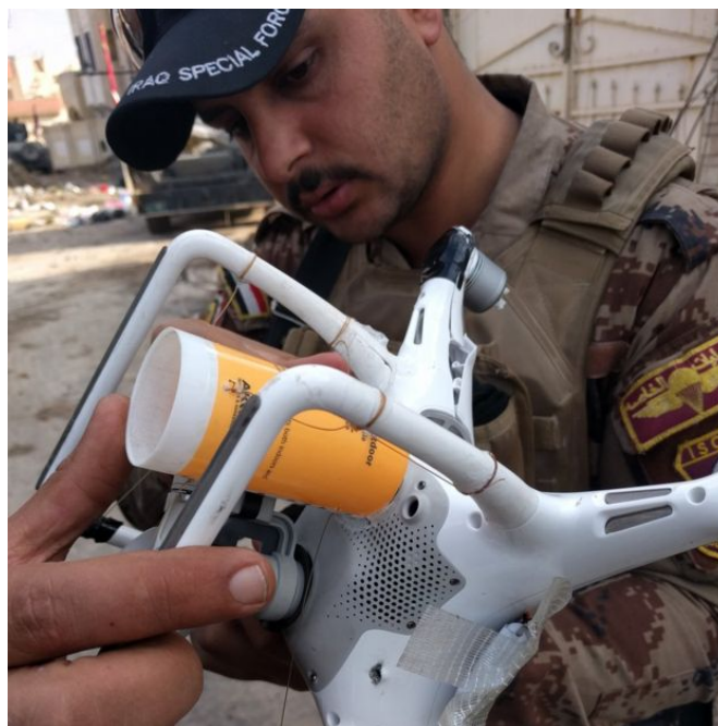
Figure 3: Basic Glue Bottle Ordnance Holder on a Captured IS Drone (Source: Mitch Utterback [14]).
