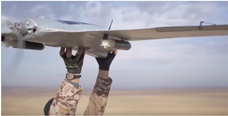
Figure 4: 8X Skywalker Drone with Two Munitions Under-Slung on its Wings (Source: Bellingcat [14]).
