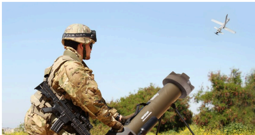
Figure 7: The Hero-30 Loitering-Munition Drone is Launched from a Pneumatic Tube (Source: UVision [24]).
