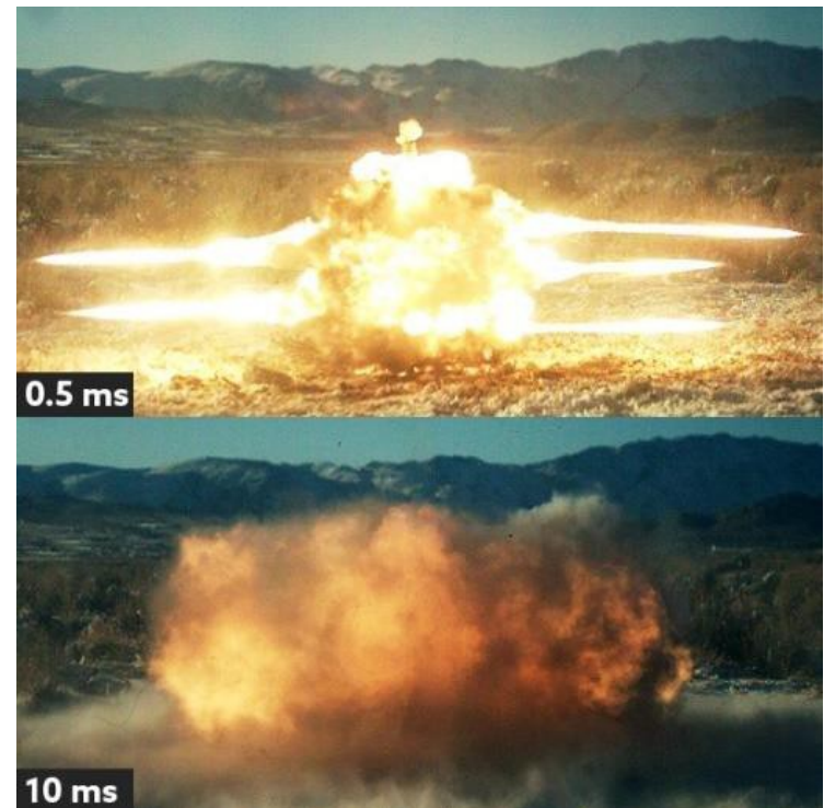
Oil tool above ground test, shaped charges fire following by GEM ignition.
