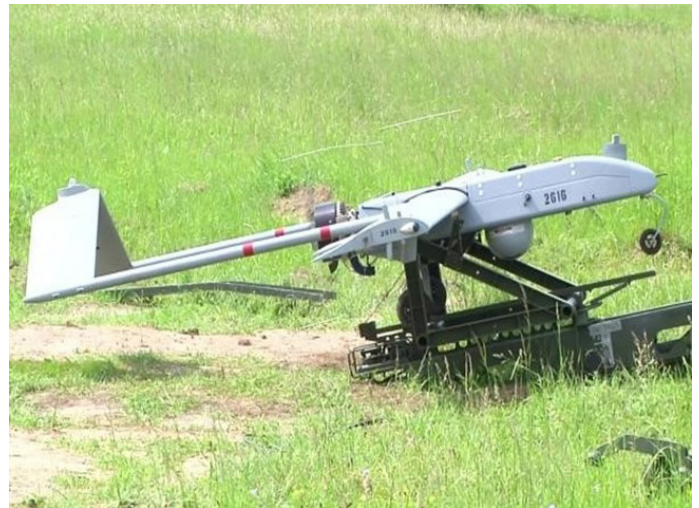
Figure 4-6. Group 2 UAV – Ground-Launched With Sensors and Gimbal for Observation and Mapping (Source: DVIDS).
