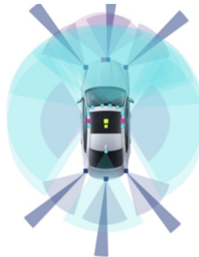
(b) Simulated, Automated Car 360-Degree Vision [4]
