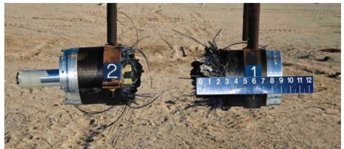
Figure 4-14. Post-Test High-Velocity FI of Motor With GIZ Propellant [54].
