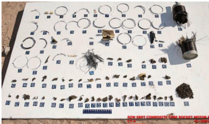
Figure 4-13. Post-Test High-Velocity FI of Motor With GIW Propellant [54].
