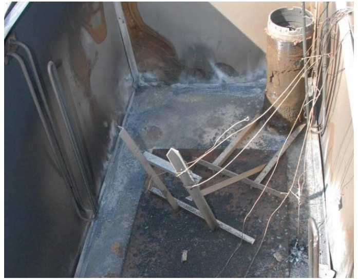
Figure 4-16. Post-Test SCO Motor With GIR Propellant, Where Motor Fell From Stand and Burned Mildly [54].
