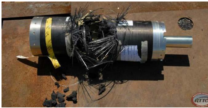
Figure 4-12. Post-Test Low-Velocity FI of Motor With GIR Propellant [54].
