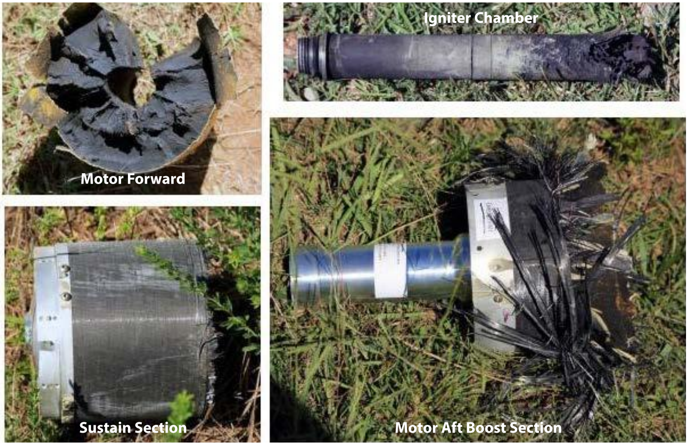
Figure 4-27. FI Post-Test Motor Without Igniter Material [55].
