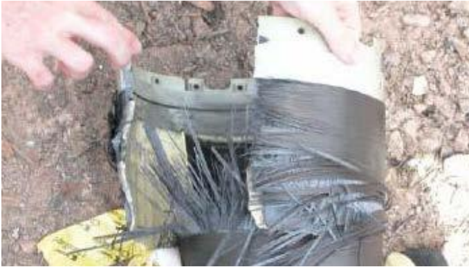
Figure 4-16. Post-Test SCO Motor With GIR Propellant, Where Motor Fell From Stand and Burned Mildly [54].
