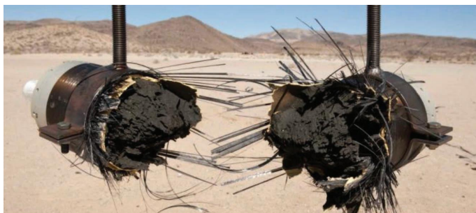
Figure 4-12. Post-Test Low-Velocity FI of Motor With GIR Propellant [54].
