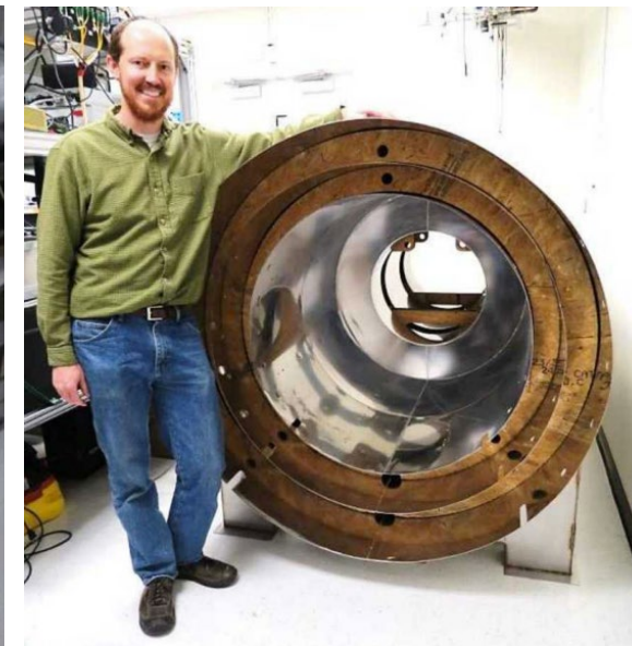
Mu Metal Enclosure (taken from osti.gov [Sandia National Labs])
