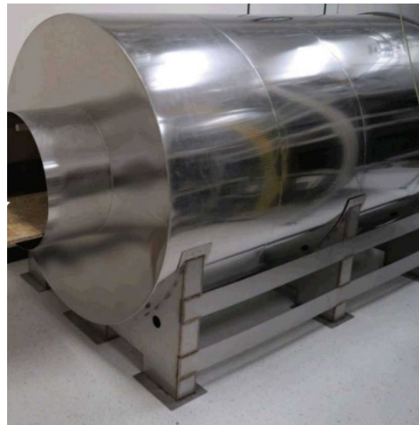
Mu Metal Enclosure (taken from osti.gov [Sandia National Labs])
