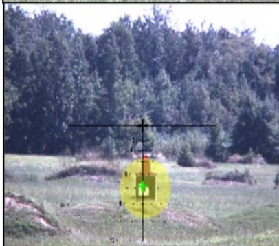
Correctly classified target, using different ATR visualization method. Aim point optimized for center mass hit, as indicated by green crosshair
