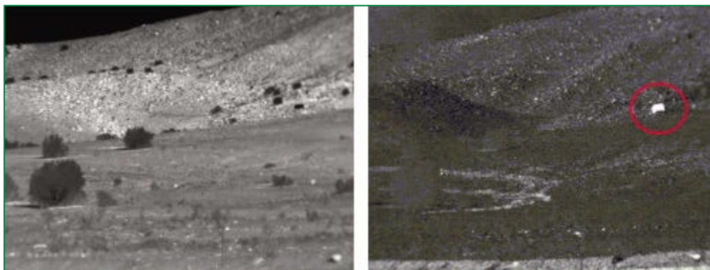
Figure 1: Example of Conventional LWIR Thermal Image (Left) and Resultant LWIR Polarimetric Image (Right) in Which a Vehicle at Ambient Temperature Is Parked on a Hillside [1].
