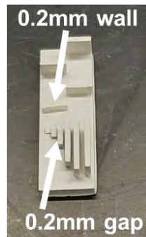
30% Platelets, Hot Pressed at 1300°C/65MPa
