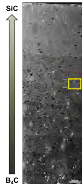
Graded SiC-B4C part with microstructure shown right
