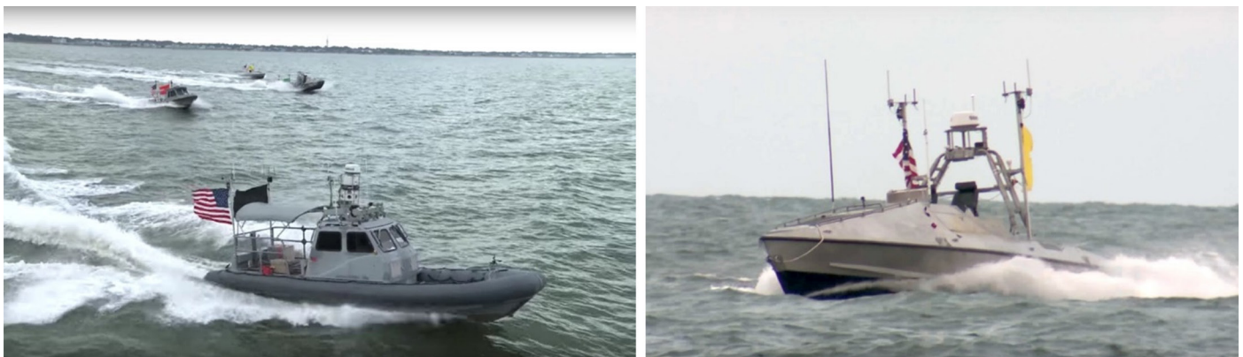
Figure 4-7. Swarm II USVs With CARACaS During Demonstrations (Source: NASA [165]).
