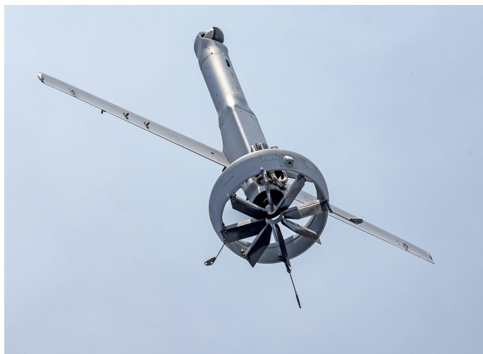
Figure 4-1. V-Bat UAV in Transition Flight From Vertical Takeoff (Source: Shield AI Used With Permission, https://shield.ai/products ).
