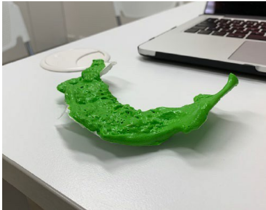
Figure 1. Warping of PLA After Autoclave Process [2].
