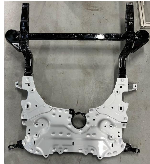
10% lighter multi-material engine cradle
